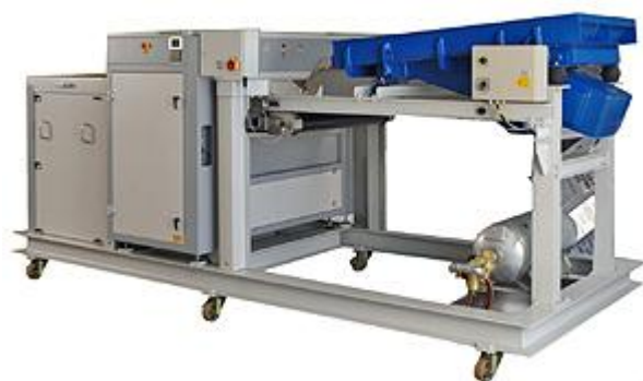
An x-ray sorting machine of the type being fitted to the Light Brothers facility
